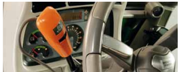
Above: Powershuttle with adjustable modulation control settings.
