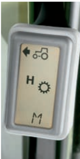
Everything in sight: The central display in the A-post shows the activated Powershift stage.
