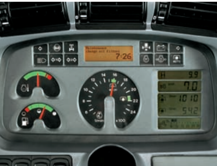
The Infocenter displays maintenance and fault messages in digital text.
