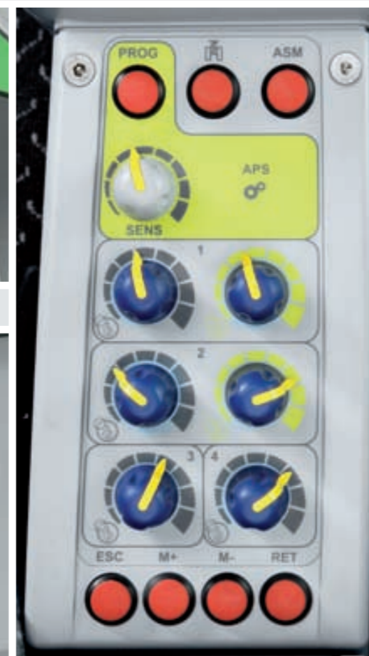
The settings of the remote valves with flow rate and time-dependent operation are conveniently adjusted with the knobs on the operating panel.
