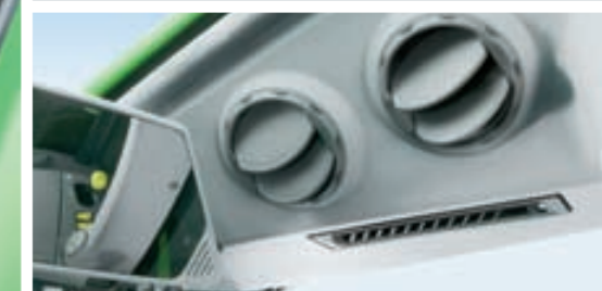
A total of 17 air nozzles ensure excellent cab ventilation and quick demisting.
