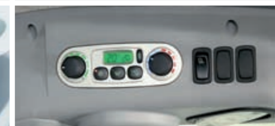
The controls for the heating and air conditioning system are installed in the roof. The air conditioning system is a standard feature of the "ProfiLine" package. An optional electronically controlled automatic air conditioner is available for the "ProfiLine" version.
