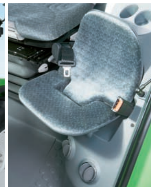
The standard co-driver seat: Upholstered, comfortable and equipped with an automatic lap belt.
