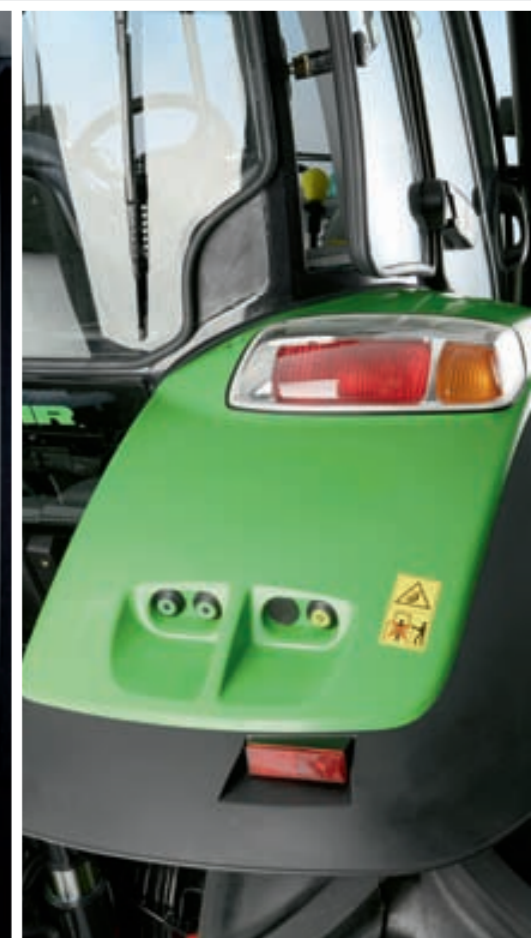
Powerlift and rear PTO can be safely operated from both rear mudguards.
