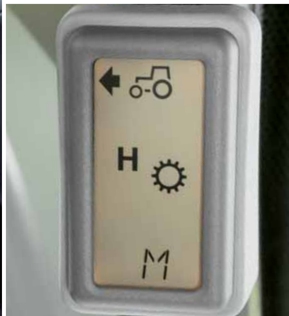
The central display in the A-post shows the activated PowerShift stage.
