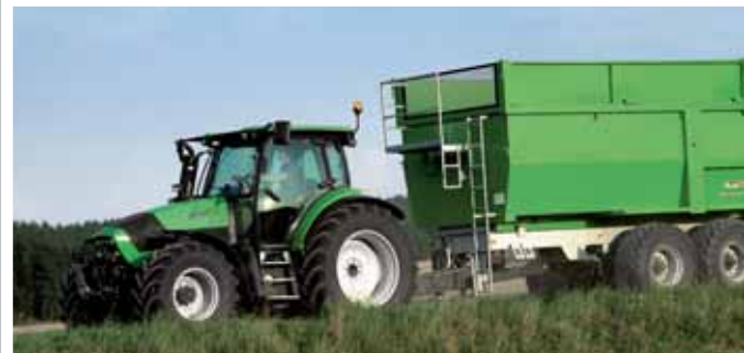
Road transport. The advantages of ASM: Speed above 15 km/h – 4wheel drive disengaged; Speed below 14 km/h – 4wheel drive engaged.
