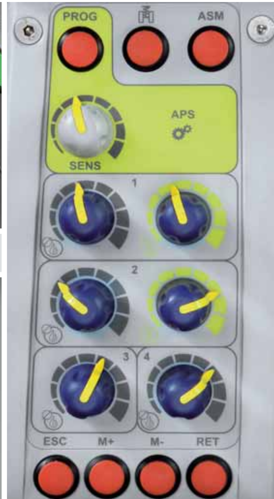
The settings of the remote valves with flow rate and time-dependent operation are conveniently adjusted with the knobs on the operating panel.
