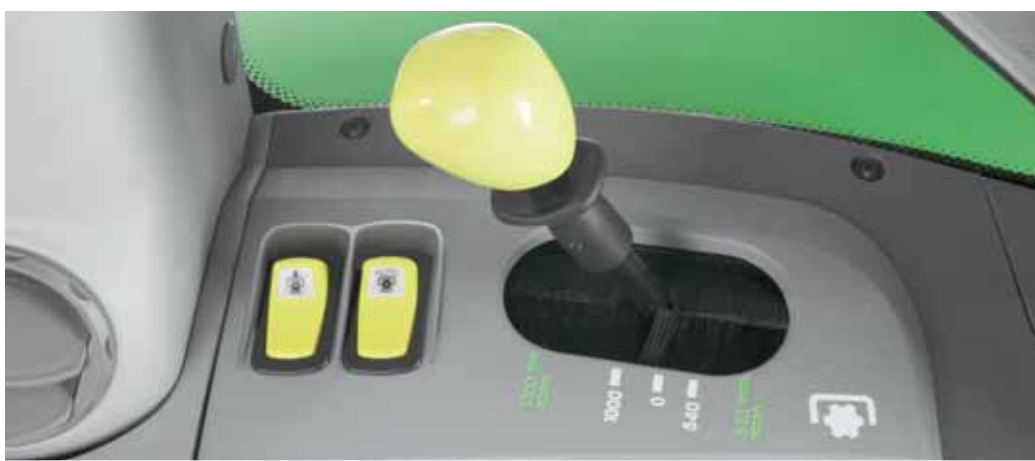
The standard four PTO speeds can be conveniently pre-selected.
