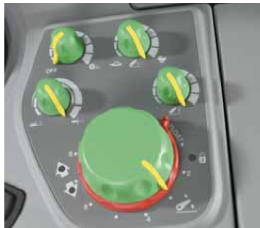
The standard EHR operating panel permits fast programming and setting adjustments.
