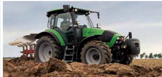
Turning in the field. The ASM principle: Steering angle greater than 15° - differential lock off; Steering angle less than 15° - differential lock on; Actuation of individual wheel brake - differential lock off.
