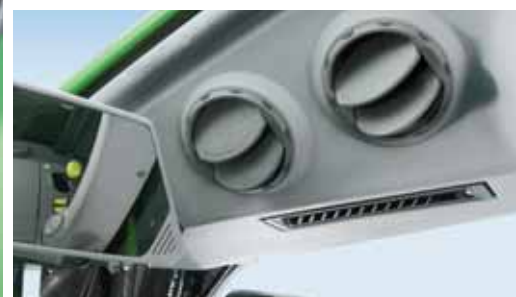
A total of 17 air nozzles ensure excellent cab ventilation and quick demisting.
