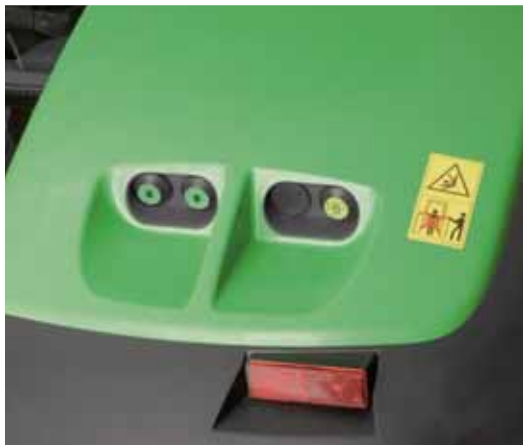
Powerlift and rear PTO can be safely operated from both rear mudguards.
