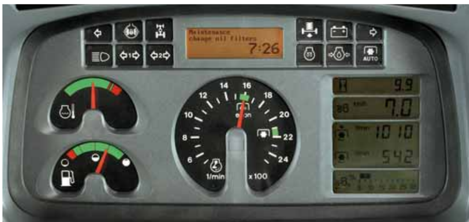
The Infocenter 3 displays maintenance and fault messages in digital text.
