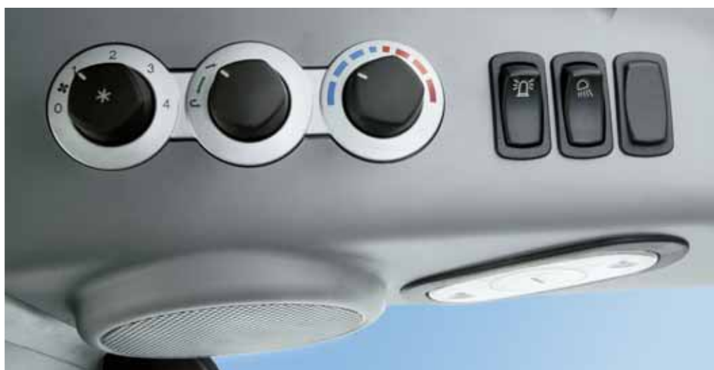
The controls for the heating and air conditioning system are installed in the roof. The air conditioning system is a standard feature of the "Profiline" package. An optional electronically controlled automatic air conditioner is available for the "Profiline" version.
