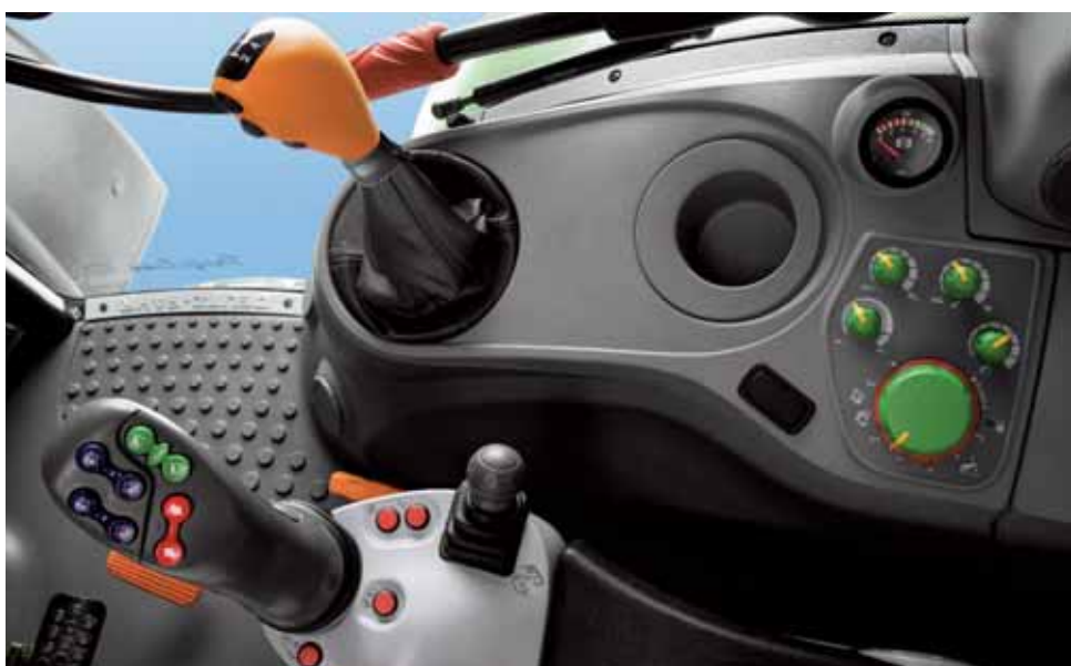
Unique in this tractor class – the new "PowerComS" armrest combines all the functions of the Agrottron K in one control unit for productive work.
