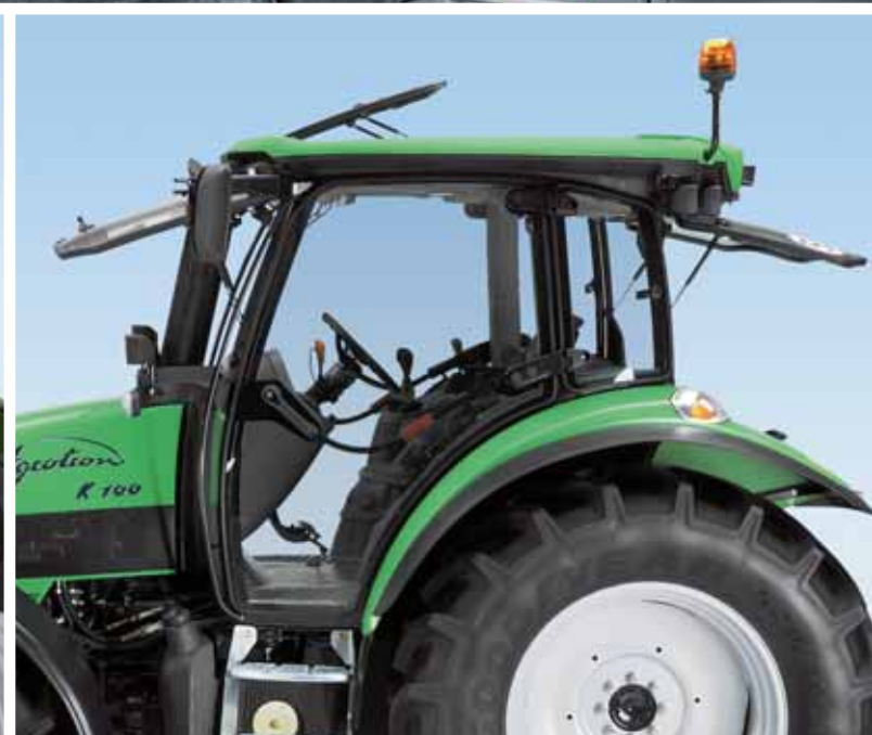
The front and rear windscreens can be opened wide. The cab also features a tilting transparent glass roof hatch that is ideal for working with front loaders.
